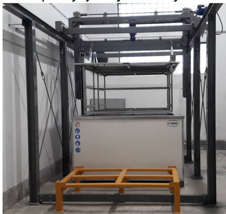
System wannowy do strippingu
